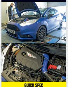
ITG induction kit, Pro Hoses induction hose, Forge Motorsport re-circ valve, KMS 3in cat-back with sports cat, ST Fabrications intercooler, Revo Stage 2 software
